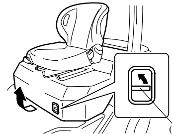
(1) Engine hood lock release lever
